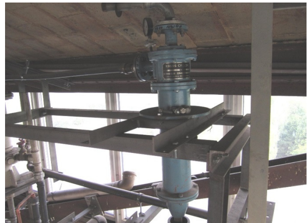
Cyclone, Krebs type D4BB-12-972, diameter 100 mm.
