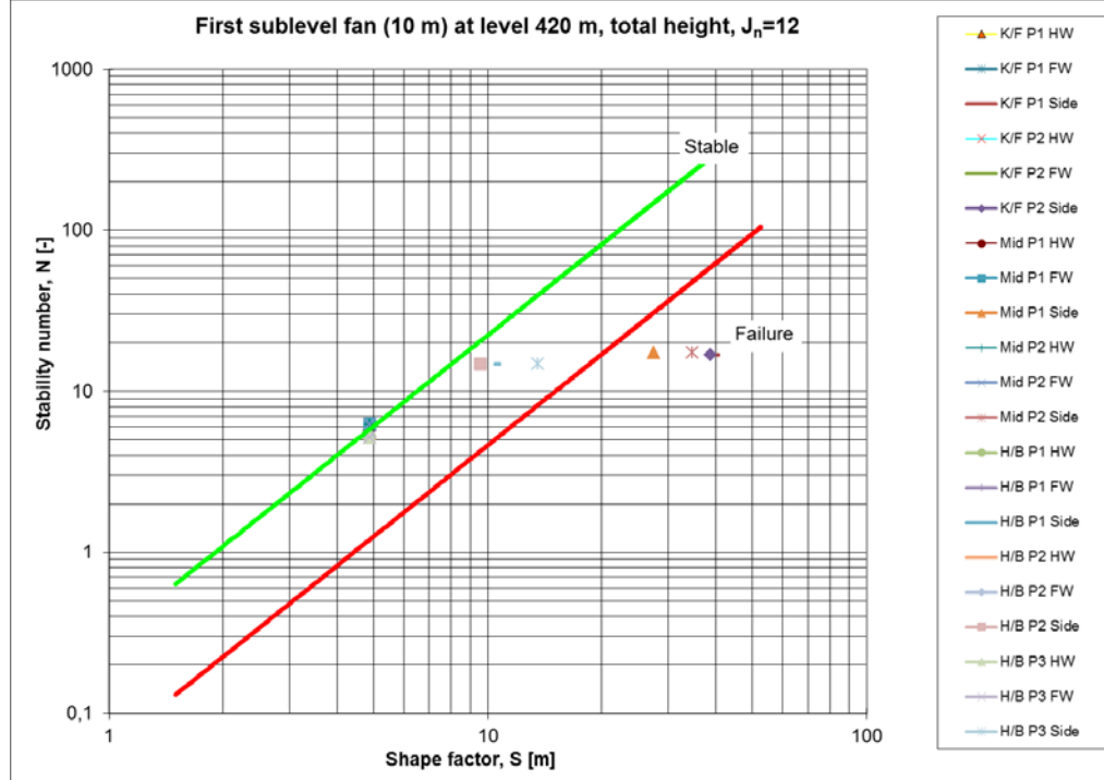
Figure 5-9 Mathews stability graph for a sublevel fan of 10m length, 420 m height and a joint set number of 12
