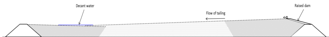
Figure 38. Potential risk with fine tailing from the ongoing spigotting flow to far over on the other side and on the coarse tailing.
