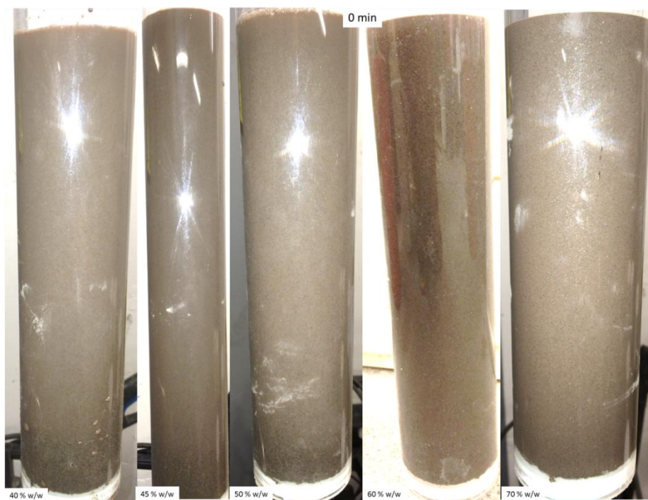
Figure 6. Vertical segregation and settling test at different solids contents tailing 1+2 at 0 min.
