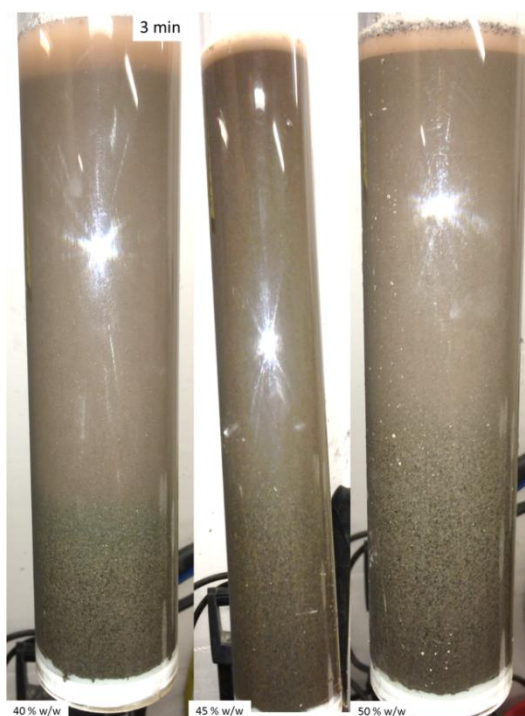
Figure 7. Vertical segregation and settling test at different solids contents tailing 1+2 at 3 min.
