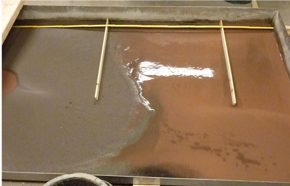
Figure 12. Result of horizontal segregation test. Coarse tailing to the left and fines to the right.
