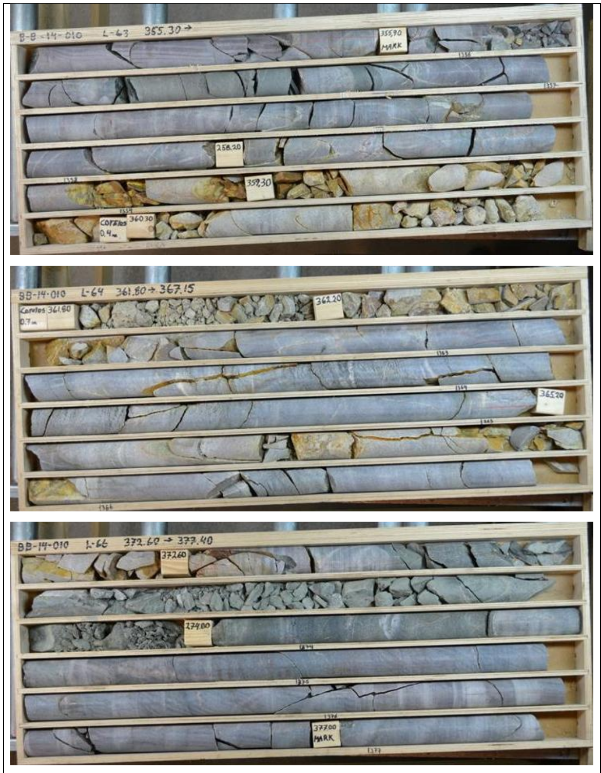
Figure 16. Sections with fractured and crushed rock in BB 14-010.
