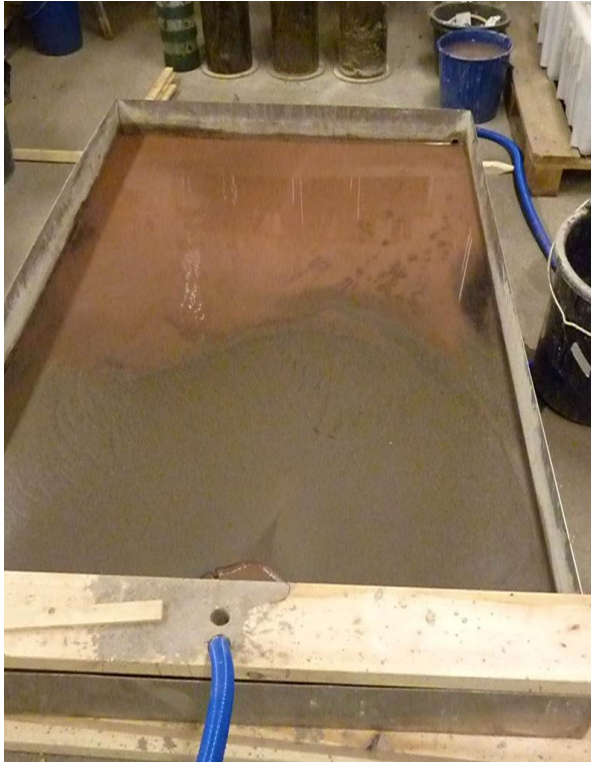
Figure 10. Flume used for horizontal segregation test. Coarse tailing at the bottom of the picture and fines at the top.
