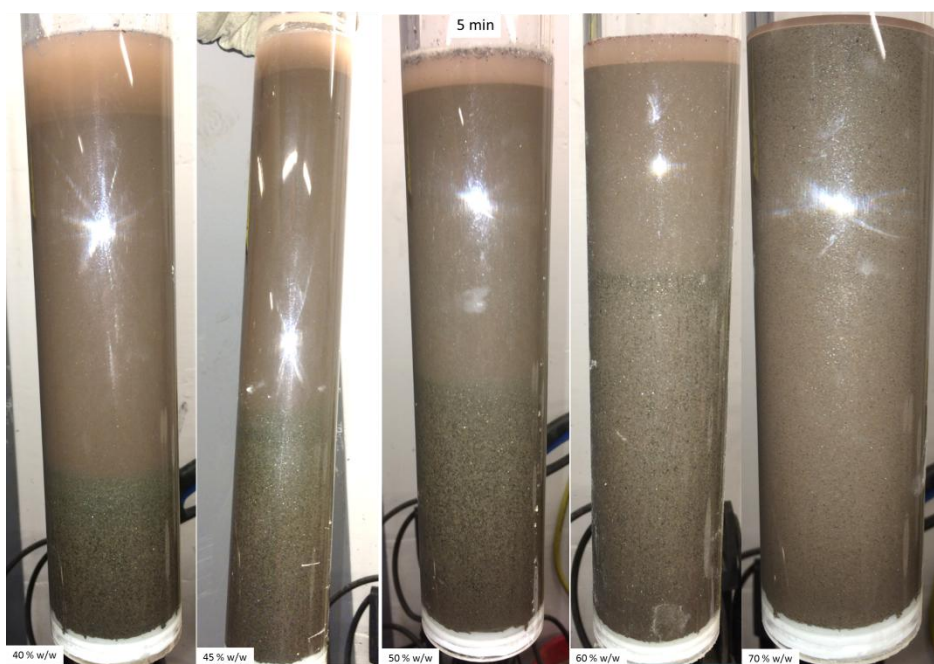
Figure 8. Vertical segregation and settling test at different solids contents tailing 1+2 at 0 min.
